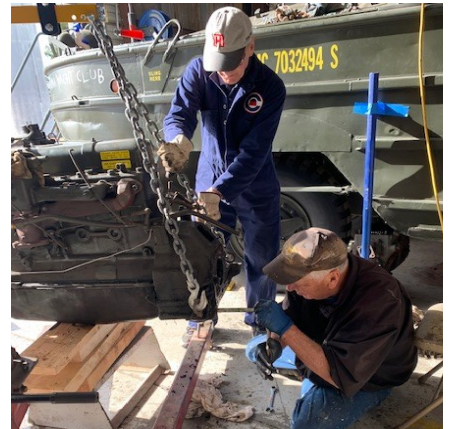
Steve Foss and Jim Brass inspect DUK Flywheel assembly
