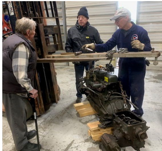
Ron Boyte, John Everett and Steve Foss inspect engine recently removed from the DUKW prior to clutch replacement
