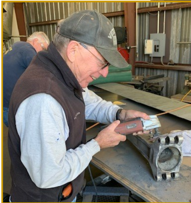
Carl Robbins Touches Up Rotor Blade I Hub with Hand Sander
