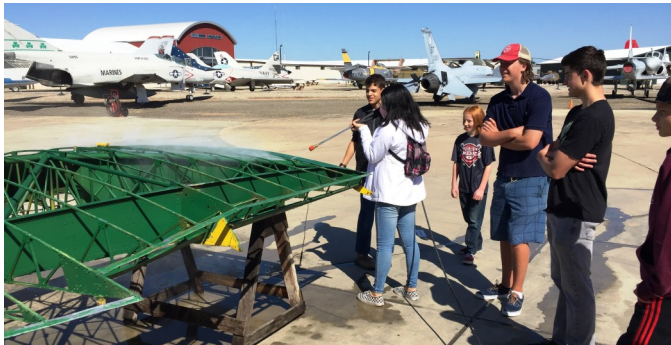
EWM Aviation Club puts the power washer to the test on Stinson starboard wing assembly. This aircraft has a fabric skin and will sport a new hide when Resto is finished.
