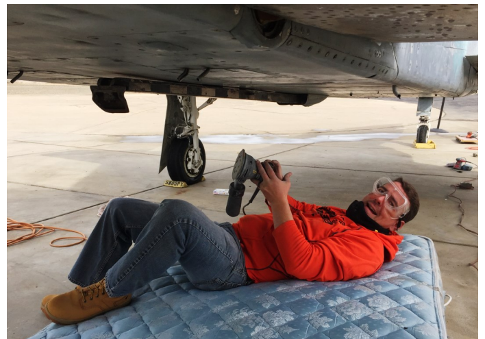
New "Resto" Elliot DePriest uses hand sander and a new Serta mattress to sand down underbelly of F-5 Freedom Fighter.
