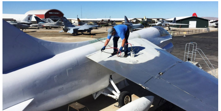
Ken applies primer to top of wing structure on the A-7 Corsair
