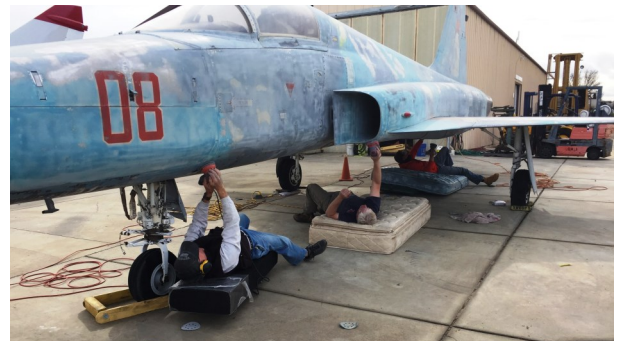
Carl Robbins, Mike Brophy and Mr. DePriest, with the help of back saving mattresses and old luggage (?) tickle (sand) the Freedom Fighter in preparation for painting.
