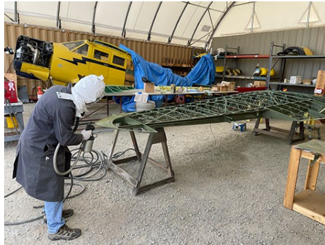
Brad Eaton, director of the EWM/PASO ROBLES/TEMPLETON AVIATION CLUB sandblasts wing strut of Stinson V-77 which the Club is currently restoring. Join the Club by calling Brad at 805-550-8755 See page 8!
