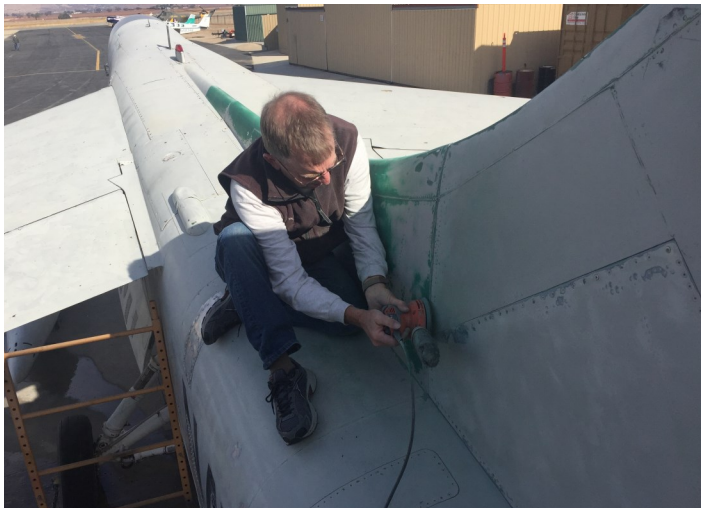
Has it been mentioned that the critical task prior to applying a $150 per-gallon of spec paint to one of our airframes (Here is Carl Robbins doing the duty on the A-7) is. . .SANDING? If you would like to lend a hand on a Monday, Wednesday or Saturday, stop by the Restoration Hangar and tell someone. Getting a job has never been so easy. Yes its taxing, but. . .it's also cool!
