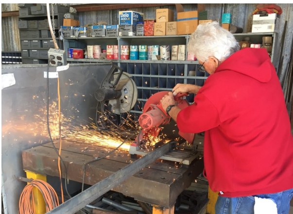
Keith Decker cuts steel reinforcing for bomb truck
