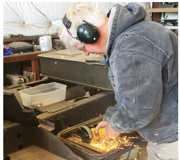
Mike Brophy grinds gas tank frame on side of Bomb Truck
