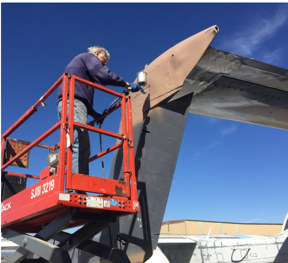
Familiar sight: Dennis Johansen applies trim coat to top section of tail assembly on the OV-10 Bronco, slated for roll-out in the near future. It will be a time of celebration as the business of Estrella/Woodland resumes in earnest!.
