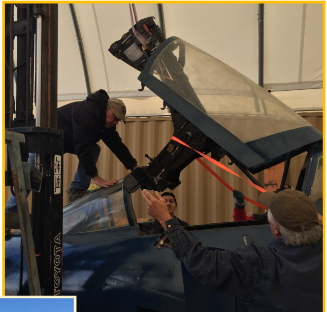
Brad Eaton guides seat into cockpit of F-4. this will end up as an interactive exhibit. Detail painting is all that is left!
