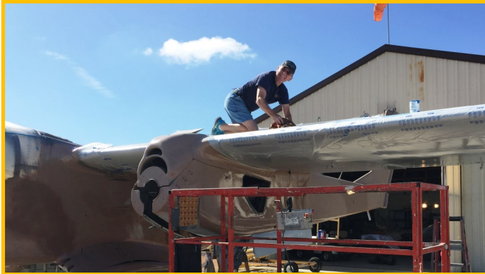
Carl Robbins tapes top of OV-10 wing for new camo paint job
