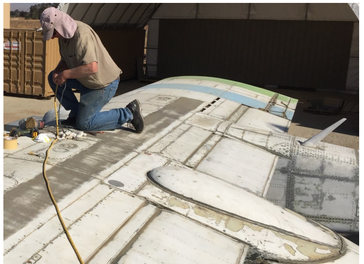
Tom DuVaul sands the OV-10 up top. This sanding is a delicate operation as the fine silica sand covers only a few fractions of an inch with each short pass.
