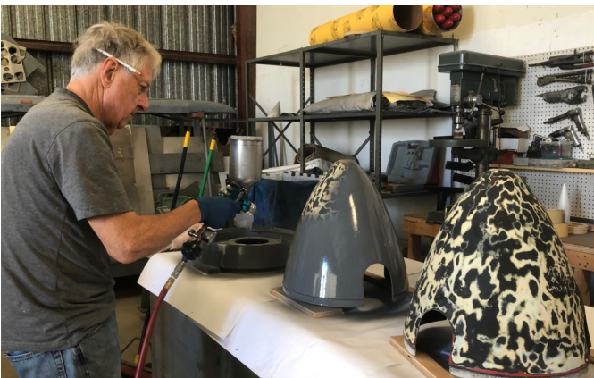
Dennis Johansen works on the prop hubs/spinners for the OV-10 Bronco.. Eventually the paint livery will match Marine specifications for aviation units in Operation Desert Storm.
