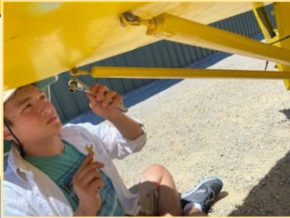
Ian Kinnear removes strut from the L-5 Stinson, which will undergo Resto Treatment starting late July!
