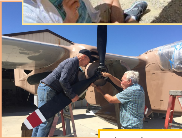
Tom Duvall and Tom Nix install starboard prop to OV-10 Bronco
