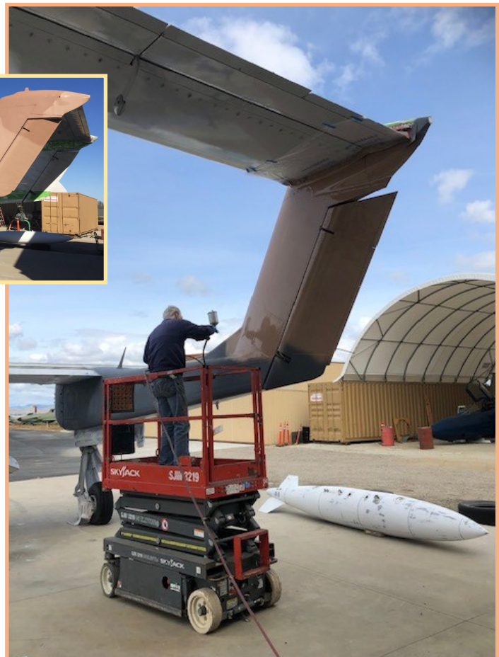
Dennis Johansen uses the lift to apply base coat of "cami" livery to the OV-10 Bronco.
