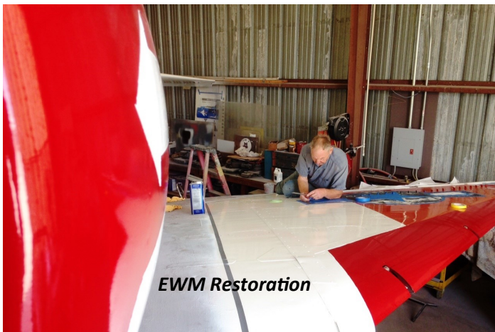
Meticulous detail in every move as Mr. DuVaul uses a razor to mask stencils over a wing panel of our TA4-J. Paint for the A4 is ordered to spec and costs about $150.00/gal
