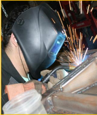
**Zach DeWeese** uses new Mig welder to patch up the floor/fender assembly of **M151A1 Jeep** with sheet metal cut and fabricated right here inside the Schade Restoration Building.
