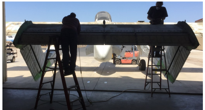
Tom DuVaul (right) and Carl Robbins sand lowered tail of OV-10 Bronco
