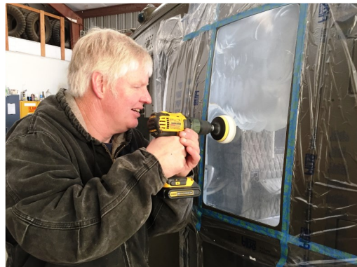
Mike Brophy leans into the side panel plexiglass on the pilot side of the UH1D. Result: Spotless.
