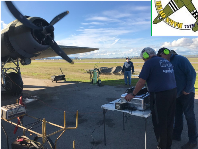
Rob Kinneer is observing (and standing by with fire prevention gear) run up and Dynamic balance test of the PORT side propeller. Operator Jeff Jefferies and Scott Stelzle monitor the gauges as prop spins.
