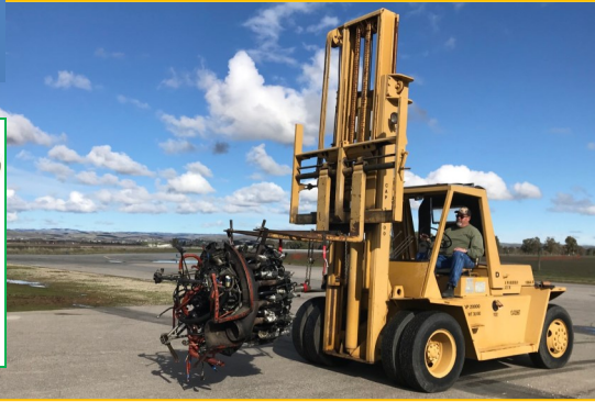
Scott Stelzle motors the new STARBOARD (right side) engine into the install area for testing/evaluation. It took the better part of a day to figure out how to best load it onto the fork for precise positioning when lifted to the exact points of attachment.
