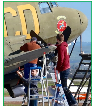
Men At Work: Scott Stelzle, son Jake (on ladder) and Aiden Bajema (Templeton HS Aviation Club members) install screws to lead edge of starboard wing prior to spin test.
