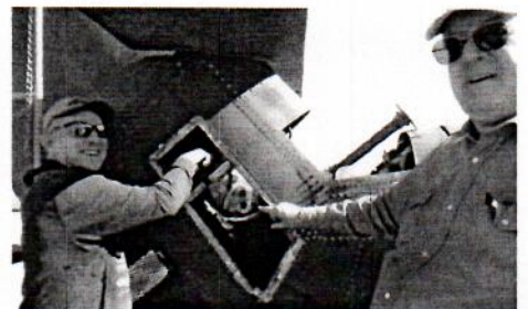
Little Tom & Big Tom inserting intermediate gear box for the H-34 tail rotor.
