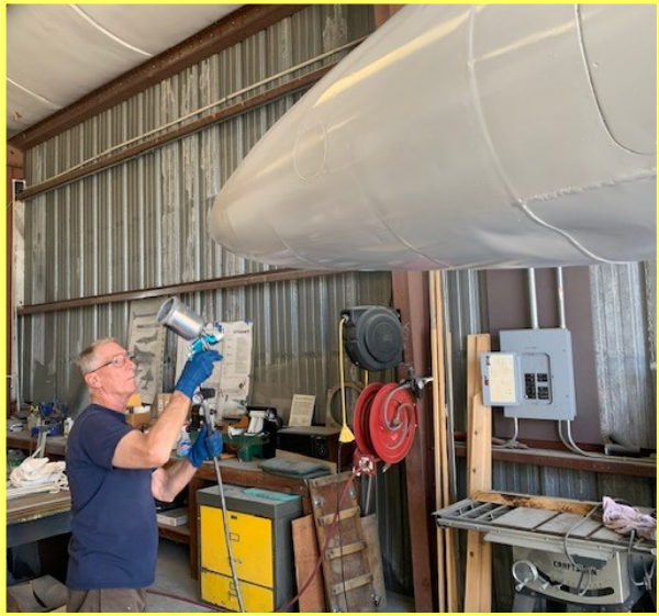
Resto Steve Foss applies finish coat to A-4's Auxiliary fuel tank, in Shade Restoration Building.
