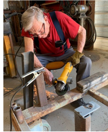
The A-7 Corsair has a new paint job. It looks like a new airplane. However the bearings in one of the wheel casings are "frozen" (they don't work) and the beast can't be rolled to its place in the outside display. A ferry/shuttle is manufactured in house to stand the plane straight and ferry it back to its display area. Here, Ron Boyte begins fabricating the wheeled ferry device which, on August 13, will be employed in the move. Stay tuned. No rest in Resto. Get dirty and help out! It's FUN!
