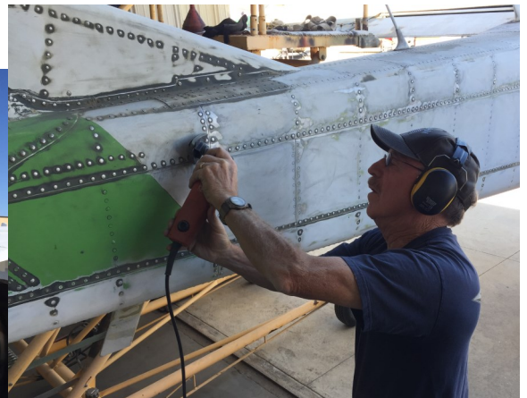
Carl Robbins carefully sands around OV-10 rivets, prior to makeup session involving primer
