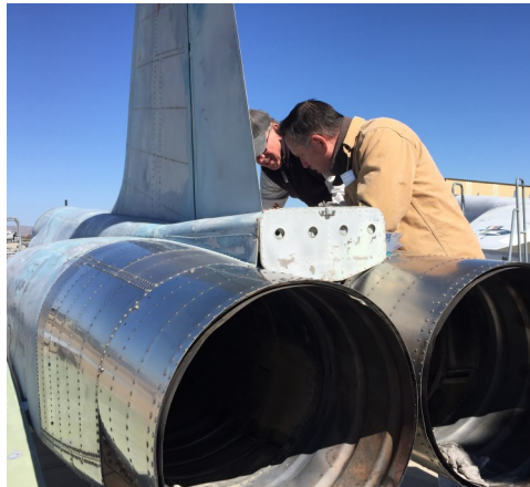
Carl Robbins and Howard Guillory tighten drag parachute dispenser on the F-5. Stuff does come loose you know.
