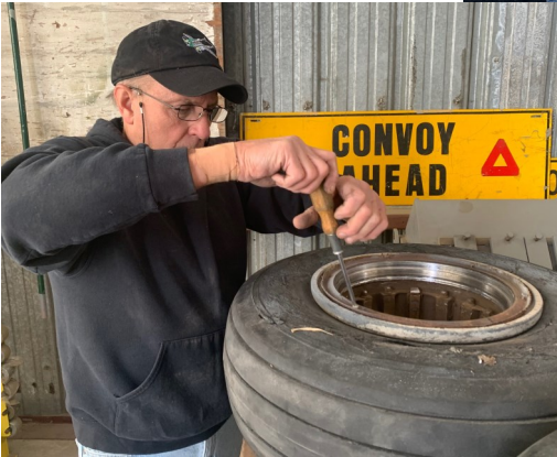
James Massineno repacks A-7 wheel bearings
